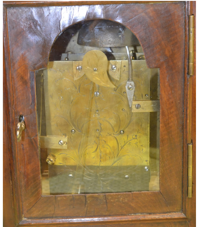
The back plate of the clock. Notice the catch for the pendulum.
